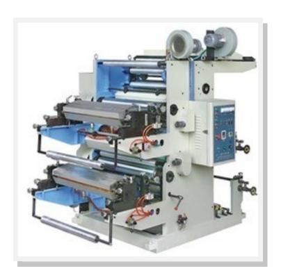
This machine uses a photosensitive resin for the printing plates, usually known as "aniline printing presses." Suitable for printing polyethylene, polypropylene plastic bags, cellophane, Web and many other packaging materials. Able to print on paper, supermarket handbags, garment bags, among others.
